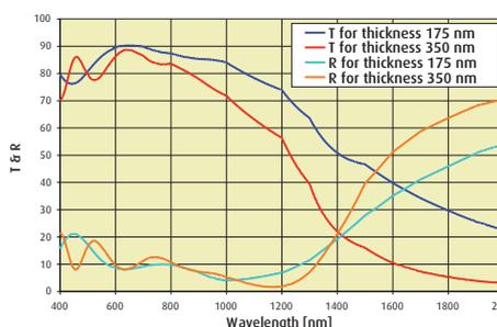
Typical transmittance and reflectance spectra for ITO.
