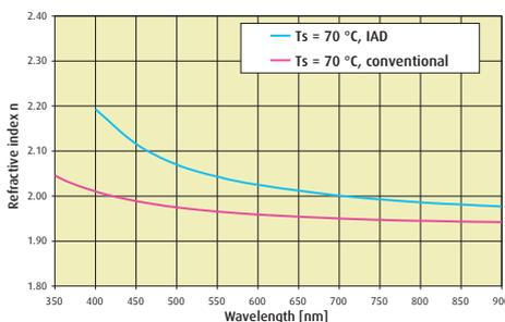
Typical dispersions of the refractive index of ZrO<sub>2</sub> films for the indicated deposition conditions. IAD parameters for coatings on plastic substrates.
