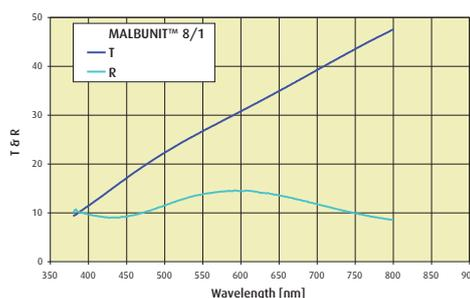
Typical transmittance and reflectance spectra for MALBUNIT™ 8/1.
