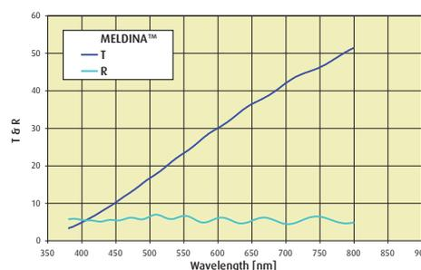
Typical transmittance and reflectance spectra for MELDINA™.
