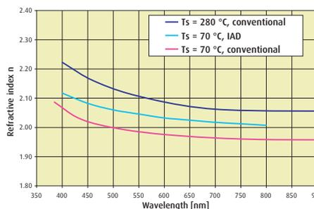
Typical dispersions of the refractive index of LATI™ films for the indicated deposition conditions. IAD parameters for coatings on plastic substrates.
