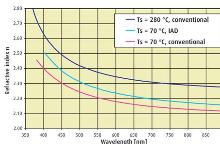
Typical dispersions of the refractive index of  $TiO_2$  films for the indicated deposition conditions. IAD parameters for coatings on plastic substrates.
