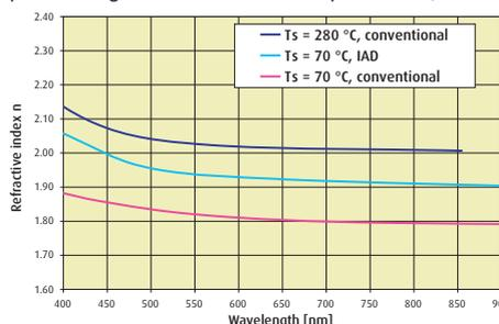
Typical dispersions of the refractive index of Zr-Ti-oxide films for the indicated deposition conditions. IAD parameters for coatings on plastic substrates.
