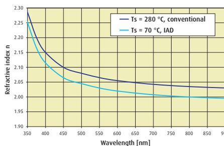
Typical dispersions of the refractive index of ROMA™ films for the indicated deposition conditions. IAD parameters for coatings on plastic substrates.
